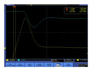
Fig.5 Reverse recovery waveforms
